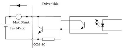
**A.** The power supply is provided by user, if the power polarity connects reversely, the drive will be damaged.
