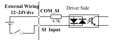
**A.** The power supply is provided by user, DC 12-24V, current  $\geq$ 100mA, if the power polarity connects reversely, the drive won't run.
