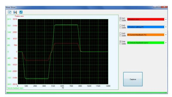
The following figure showing Pr0.02=2, Pr0.03=70, the position error (curve in red) is unacceptable! Keep decreasing value of Pr0.03, then the position error become smaller and smaller.
