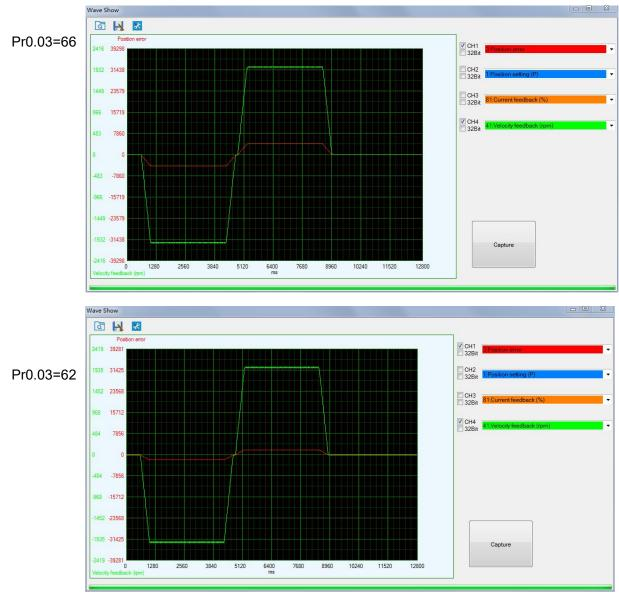
As keep decreasing the value pf Pr0.03, the position loop gain Kp become bigger and bigger, the integration time constant Vi become smaller and smaller, the position error become close to zero. Pr0.03=61
