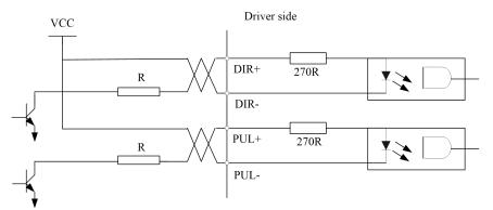
Wiring method of 24V single-ended signal (Pin 4/6/16/17)
