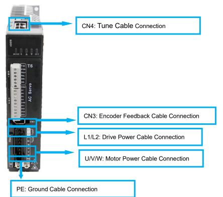
1.1.2 Connect to tune software. (Perform this step if it is necessary to install driver)
