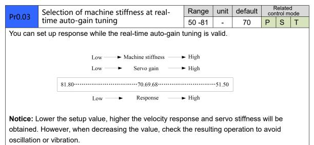
Control gain is updated while the motor is stopped. If the motor can't be stopped due to excessively low gain or continuous application of one-way direction command ,any change made to Pr0.03 is not used for update. If the changed stiffness setting is made valid after the motor stopped, abnormal sound or oscillation will be generated. To prevent this problem, stop the motor after changing the stiffness setting and check that the changed setting is enabled.
