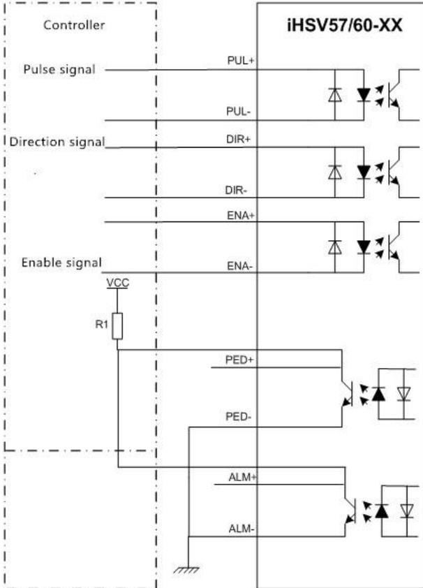
Note: VCC is compatible with 5V~24V. The resistance R1 is connected to the control signal terminal, and the resistance value is 3~5K.
