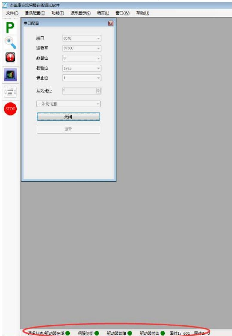
**Note:** If the connection is not available, please confirm whether COM port is selected correctly, whether the communication line is connected properly, and then reconnect according to the above steps. **Click the upper left option P**
